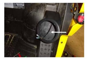
After securing the allen bolts with the 7/16 nuts run your speaker wire into the kick panel
