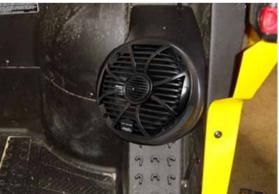
After attaching the speaker wires to the speaker install the speaker into the Wet Sounds kick panel after the 4 screws are secured secure the grill over the speaker
