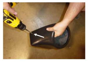
Drill a hole in the top of each kick panel, this is where the speaker wire will run out of. Sealing this hole will give you better sound from the speaker
