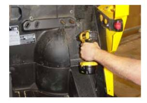
After marking the holes, drill the mounting holes using a 1/4" drill hit
